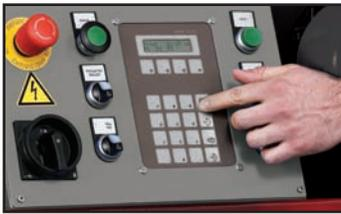
The PackTiger® system features an easy-to-use control panel that stores up to 24 custom pad configurations. In manual mode, creating pads is as simple as pushing a button or foot pedal. The PackTiger® system can also
