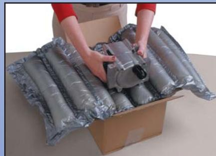
3. The operator centers the product on the tubes, setting both into the carton.
