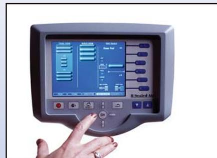
1. With the easy-to-use control panel, the operator selects the number of tubes, their thickness, and length.
