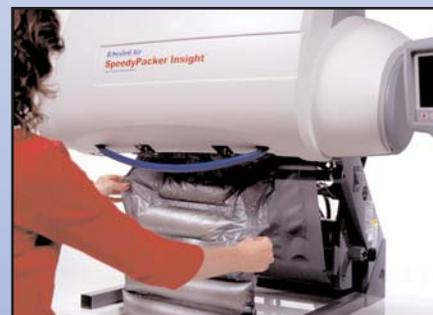
2. The system dispenses the desired amount of continuous foam tubes.
