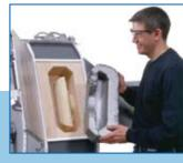
3. After the cushion has fully expanded, it is removed with the help of a built-in air ejection system.
