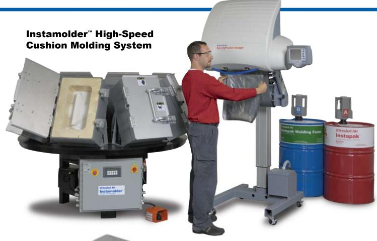
The Instamolder™ system can produce up to 600 protective cushions an hour, ideal for high-volume operations. The unit comes in 8, 10 or 12 mold box configurations and only requires 50 square feet of floor space.
