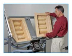
• **Tooling** – When you are ready to implement your new Instapak® molded solution, Sealed Air will manufacture custom-made production tooling ready for installation.
