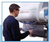
With the push of a button, the SpeedyPacker Insight® system quickly dispenses an Instapak® foam-filled bag.
